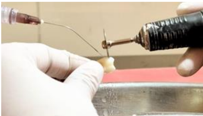
Sectioning of samples at the level of CEJ using a diamond disk under water coolant
