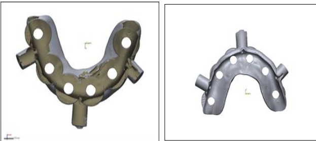
Cameo and Intaglio Surface of the Measured Data (DLP PRINTED - D2) Surgical Guide in Geomagic
