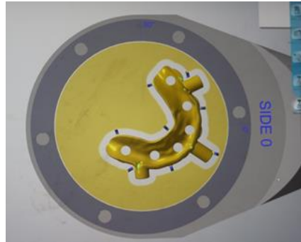
Figure 5: Orientation of PMMA Disc in Blank Holder
