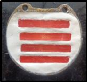
Figure 2: Flasking of wax strips
