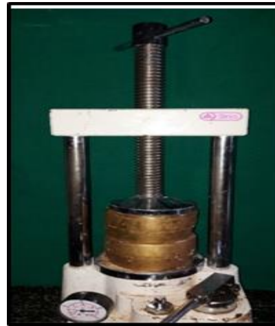
Figure 4: Packed flask under hydraulic bench
