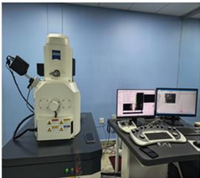
Figure 1: Scanning Electron Microscope (ZEISS EVO 18, Germany)
