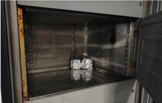
Figure 5: Storage of mixed Polymethylmethacrylate resins in airtight plastic containers covered with aluminium foil kept in deep freezer
