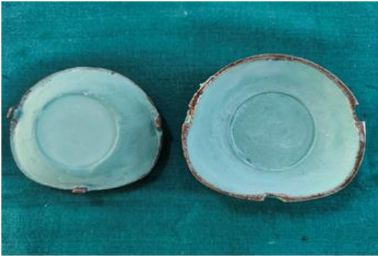
Figure 4: Mould of acrylic disc invested in dental stone
