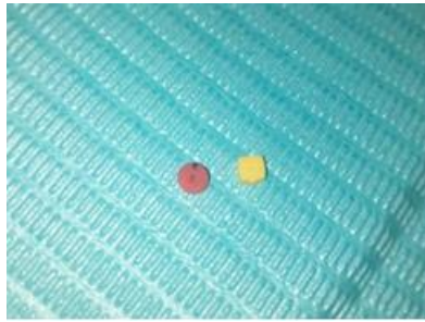
Figure 14: Rubber discs used to create areas of suction in reservoir
