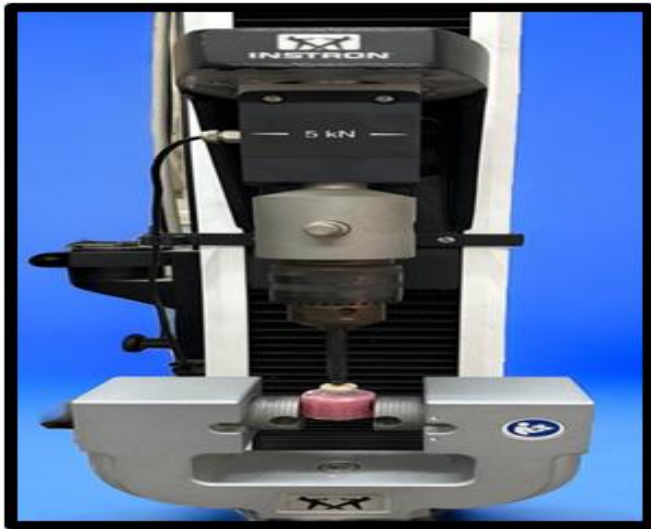
Figure 4: Instron® Bluehill Lite Software equipped with a 5 KN load cell.
