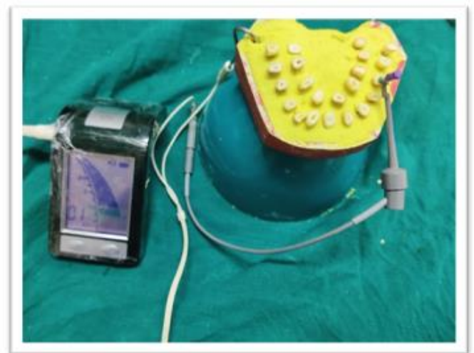
Figure 1: Roots Fixed Into A Alginate Based Custom Made Models And The Root Zx Mini Lip Clip Also Fixed In The Model.
