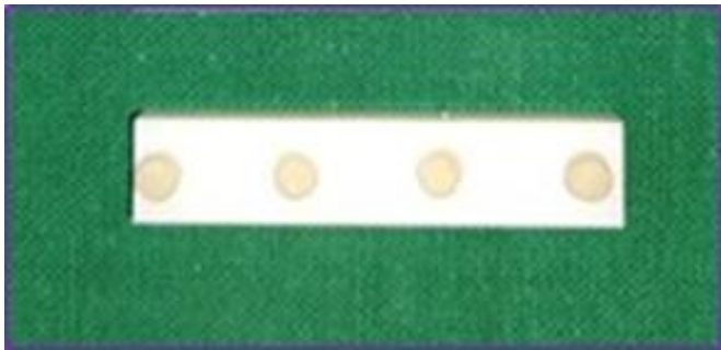
Fig. 1: Resin stubs bonded on zirconia substrate.
