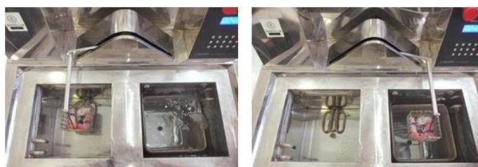
Figure 8: Thermocycling of samples for delayed testing
