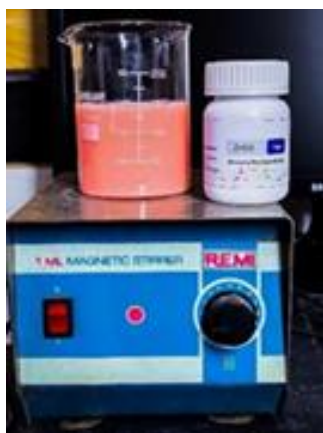
Figure 5: 1wt% Zirconium oxide nanoparticles reinforced 3D printed PMMA preparation
