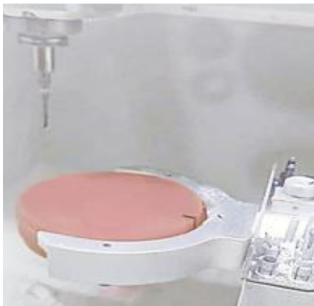
Figure 2: CAD CAM specimen preparation
