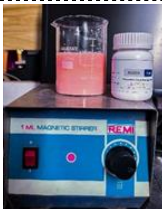
Figure 4: 2.5wt% Aluminium oxide nanoparticles reinforced 3D printed PMMA preparation
