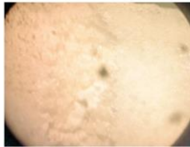
Figure 6: Showing Hydroxyapatite (HA)-coated implant under optical
