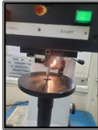
Figure 3: Knoop Hardness Testing Procedure
