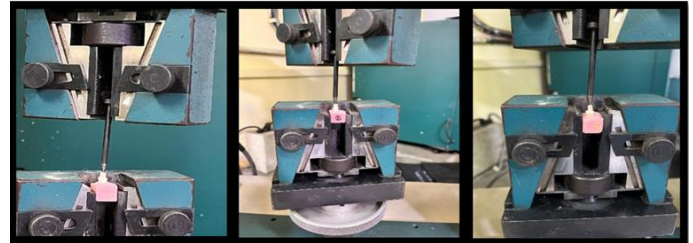
Figure 1: Testing of samples under Universal Testing Machine
