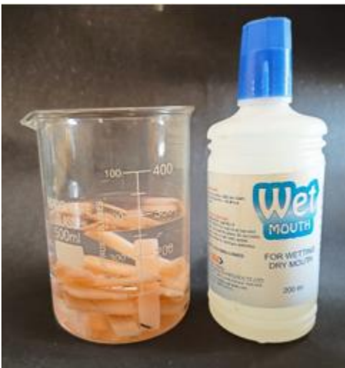
Figure 8: All specimens were placed in artificial saliva for 2 weeks before testing of samples
