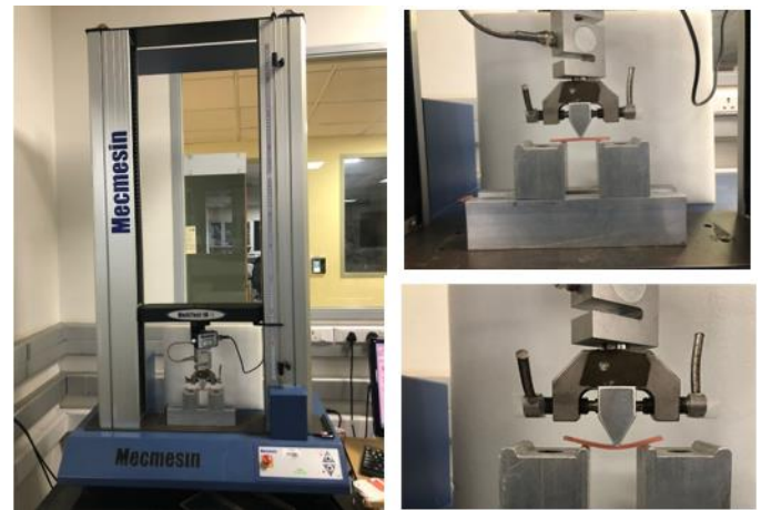
Figure 9: Three-point flexural test using universal testing machine.
