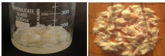
Figure 3: Bamboo fibres soaked in 6% NaOH for 12 hours and dried under sun for 2 weeks
