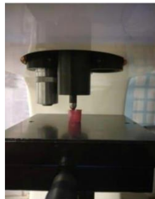
Figure 1: Dentin microhardness determination in each specimen with a Vickers hardness tester
