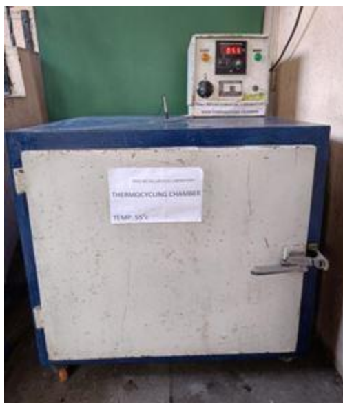
Figure 5: Thermo cycling Chamber at 55°C.
