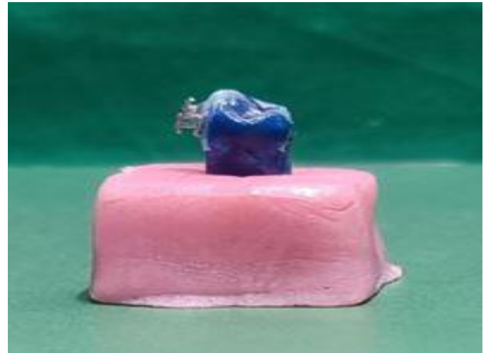
Figure 6: Bonded tooth embedded in acrylic block.
