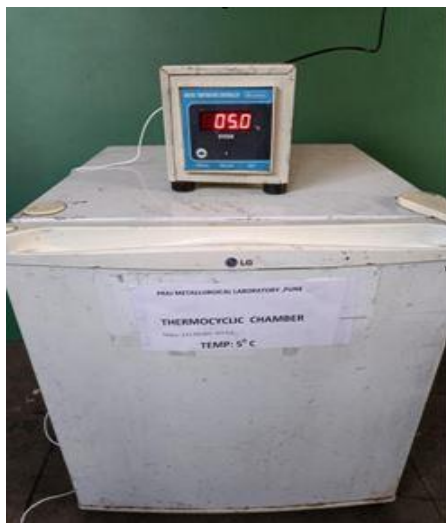
Figure 4: Thermo cycling Chamber at 5°C.
