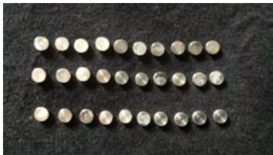
Fig12: Titanium discs 5mm in diameter and 2mm in width used in the study
