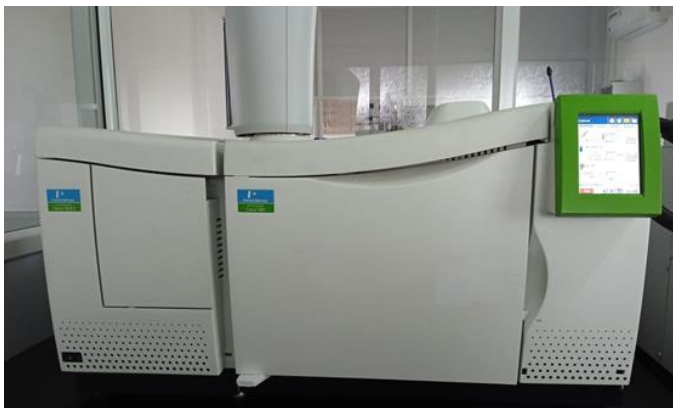
Figure 8: Gas Chromatography and Mass Spectrometry (Clarus 680 and Clarus SQ 8C)
