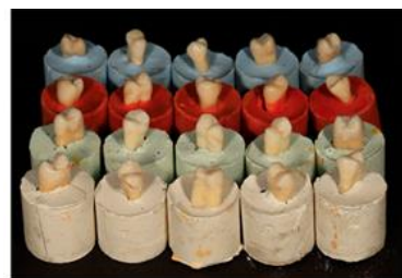
Figure 1: Prepared samples embedded in color-coded plaster blocks for shear bond strength testing. Each color represents a different adhesive group.
