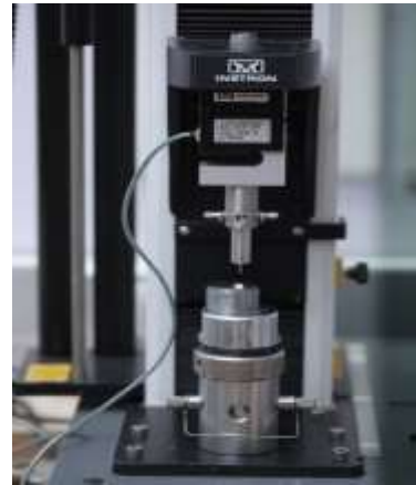
Figure 8: The universal testing machine (Instron India Pvt., Ltd.) with the stainless steel indenter of 1 mm tip diameter.
