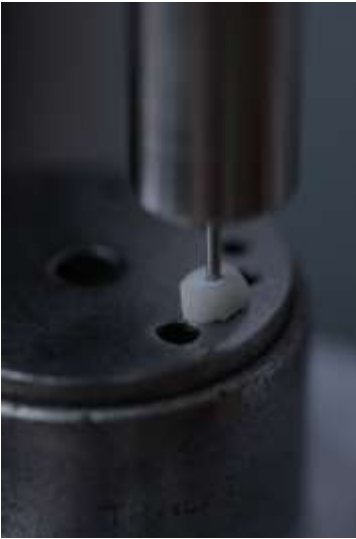
Figure 10: The custom-made base with a hole on which each sample was placed
