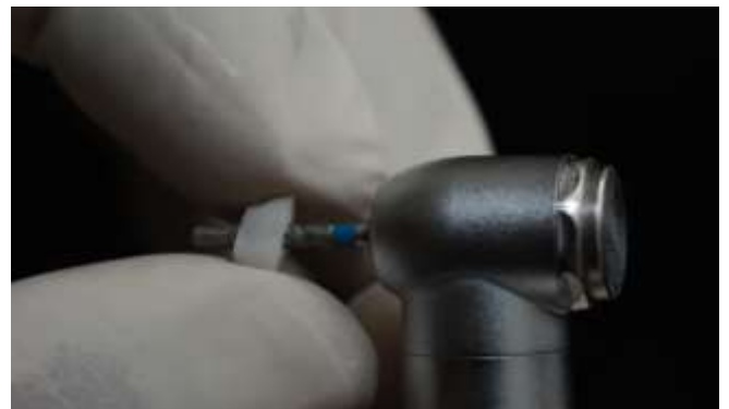
Figure 5: Canals of all the 2mm dentin sections were enlarged to a standardized cavity size of 1.3mm diameter using SF 31 straight bur (head diameter 1.3mm)
