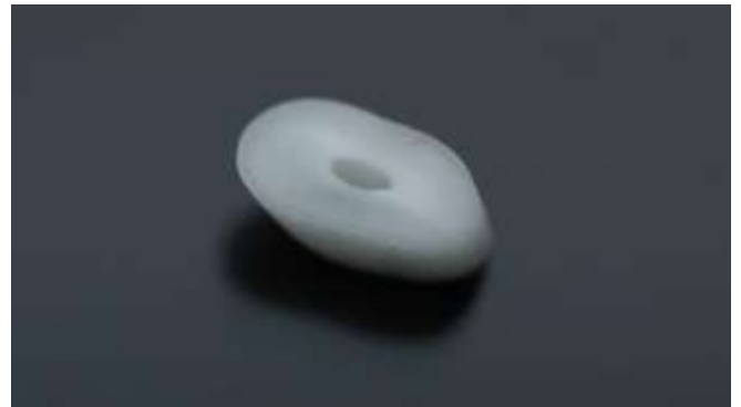
Figure 4: The 2mm thickness slice from the apical side of the remaining root of each tooth, cut with a water-cooled low-speed diamond saw (Isomet; Buehler, Lake Bluff, NY, USA) perpendicular to the long axis of the root.
