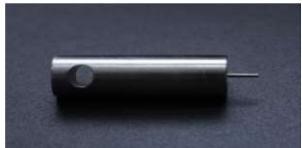
Figure 9: The stainless steel indenter with 1mm tip diameter
