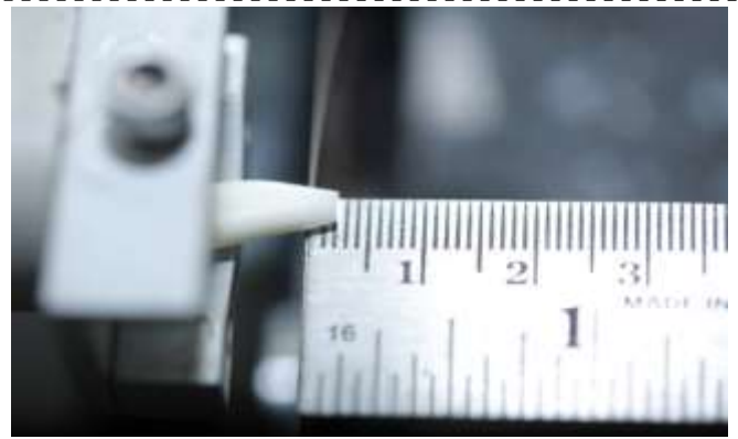
Figure 3: A 2mm thickness slice from the apical side of the remaining root of each tooth was cut with a water-cooled low-speed diamond saw (Isomet; Buehler, Lake Bluff, NY, USA) perpendicular to the long axis of the root.
