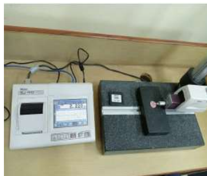
Figure 5: Surfcoader measuring surface roughness
