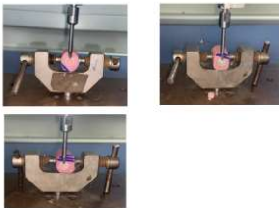
Figure 7: Shear Bond Strength Testing of Group 1, Group 2a and Group 2b Specimens
