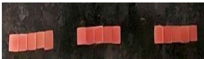
Figure 6: 15 Injection molded heat cure PMMA samples of dimensions 10*10*2mm were obtained after acrylisation
