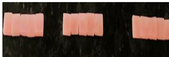
Figure 3: 15 Compression molded heat cure PMMA samples of dimensions 10*10*2mm were obtained after acrylisation.
