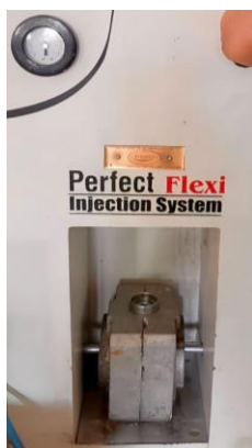
Figure 5: The wax patterns were flaked, followed by dewaxing, packing with heat cure PMMA using the SR Ivocap Heat-Cure injection system, and acrylising using the Perfect Flexi and Acrylic Injection System
