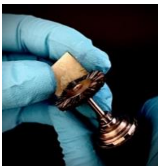
Figure 19: High gloss polishing using renfert cotton buff coated with renfert diamond polishing paste
