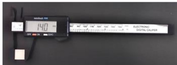
Figure 3: Digital Calipers Demonstrating the Dimensions of the Monolithic Zirconia Samples (14*14*2 Mm)
