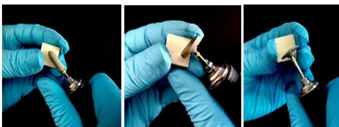
Figure 22: Finishing using the shofu zilmaster medium bur
