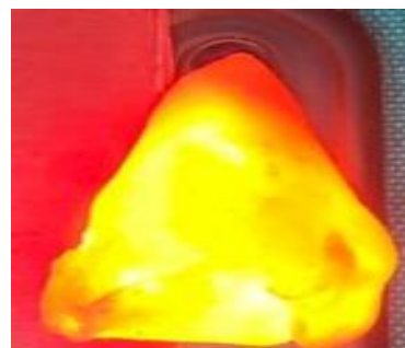
Figure 9: Self Cure Cone In Flashlight To Check Its Hollowness
