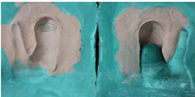
Figure 7: Mold obtained after dewaxing the wax Pattern
