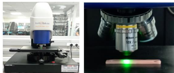
Figure 6: An optical profilometer was used to measure the abrasion resistance.
