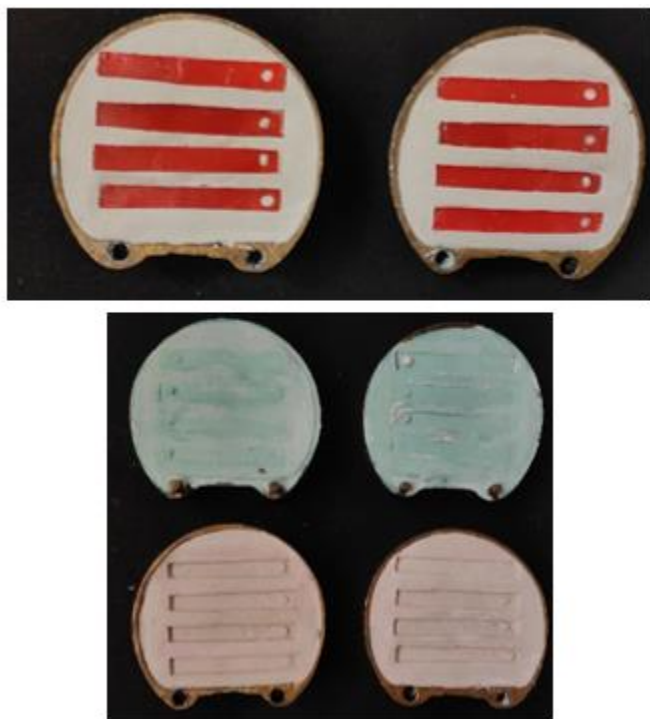
Figure 2: Wax Patterns were flaked, dewaxed, packed and acrylized with heat cure PMMA.
