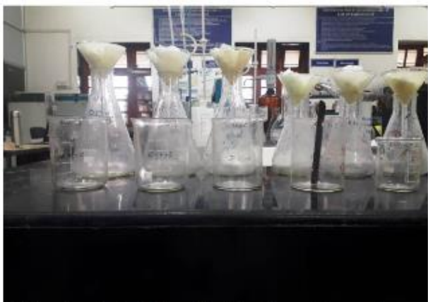
D. Preparation of carrier solution and dissolution of facemask for spectrophotometry
