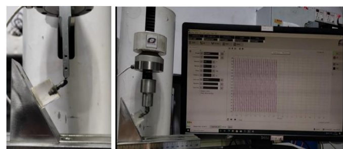
Fig. 10: Cyclic load of 50N to 350N at 15 Hz up to 10,00,000 cycles were applied.
