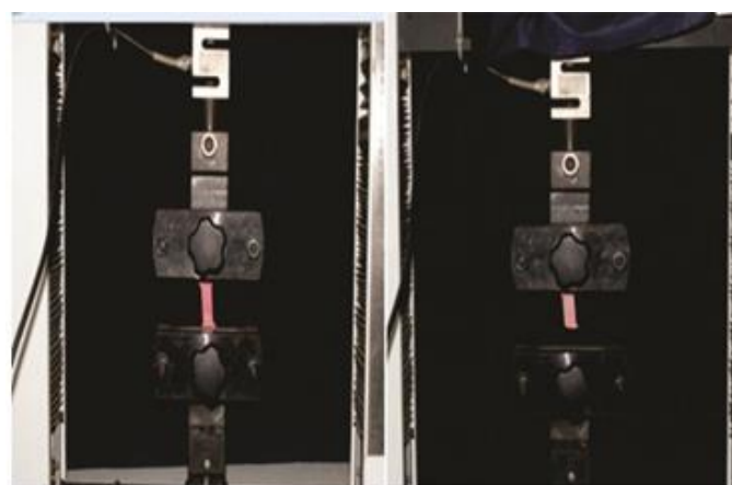
Figure 8: Specimens tested in Universal Testing Machine
