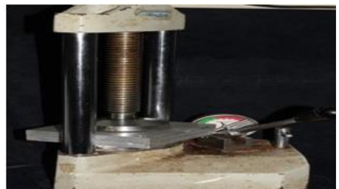
Figure 2a : Customized die placed under Bench Pressing machine
