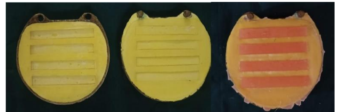
Figure 3: Heat-polymerized acrylic resin packed in the flasks after dewaxing
