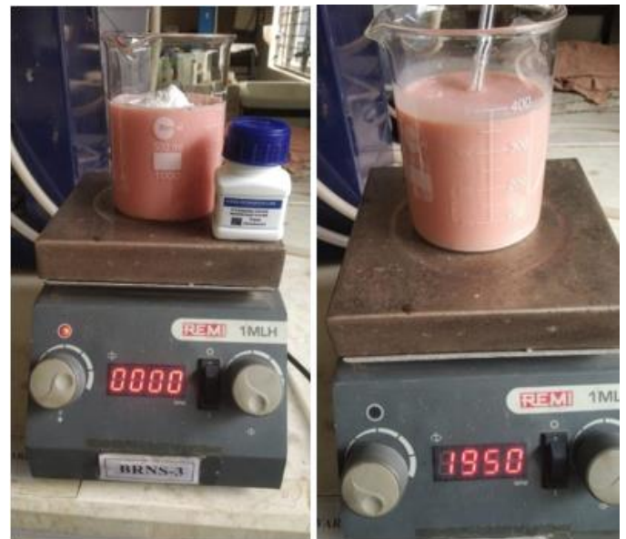
Figure 6: Resin with added TiO 2 nanoparticle was magnetically ultrasonicated stirred
