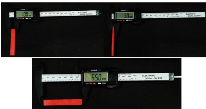
Figure 1: Wax pattern of the specimens with dimensions of 65*10*3 mm
