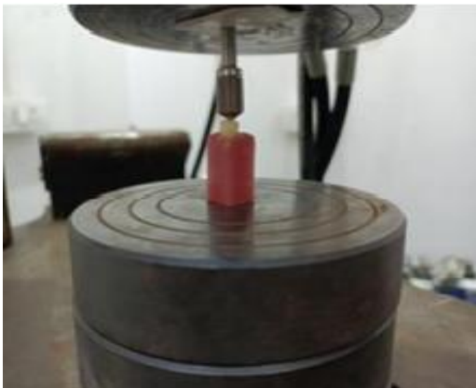
Figure 4: Fractured tooth with fiber post.
