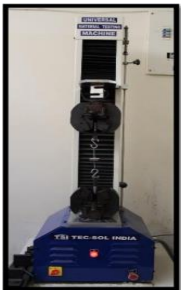
Fig 5: Test assembly loaded onto the universal testing machine.
