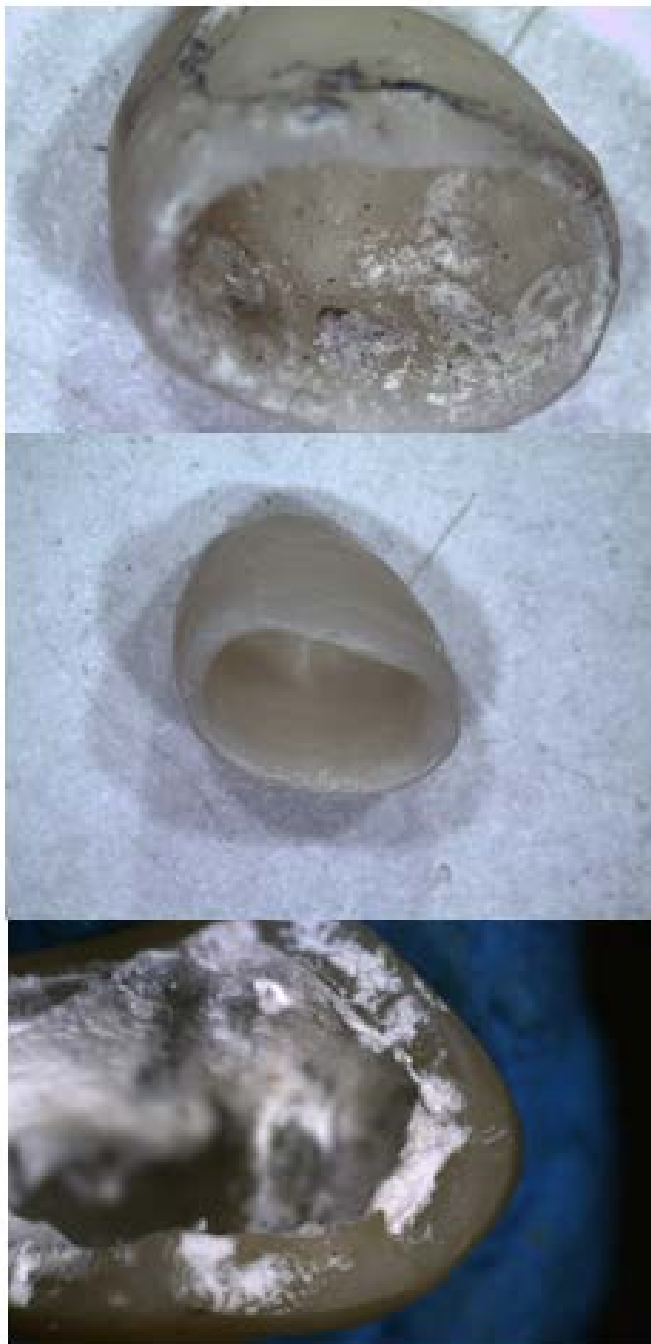
Figure 11: Cohesive, Adhesive, Mixed fracture mode
