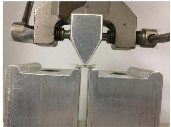
Figure 8: 3 point bending test
