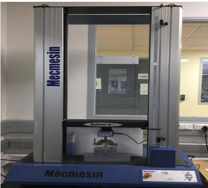
Figure 7: Universal Testing Machine (Mecmesin)
