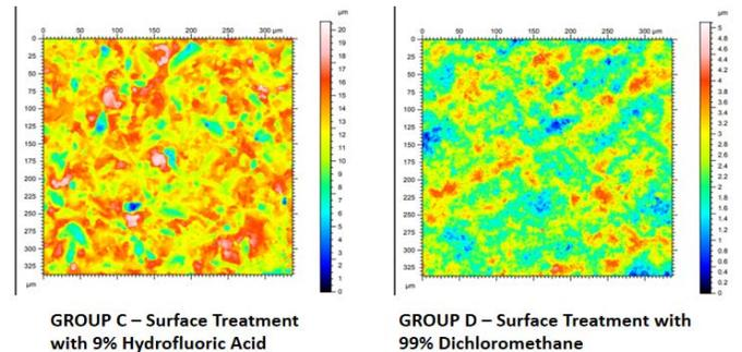
Figure 6: Surface roughness of Group C and D
