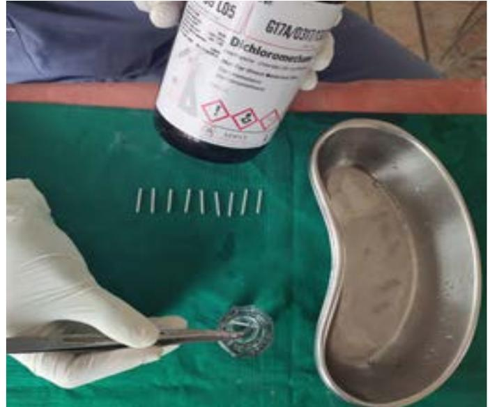
Figure 4: Treatment with 99% Dichloromethane
