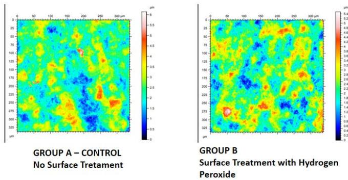
Figure 5: Surface Roughness of Group A and B
