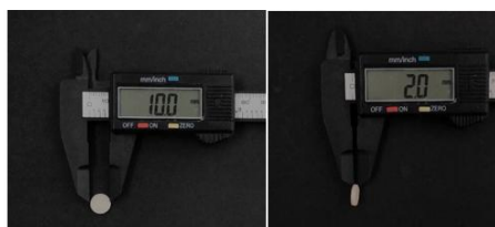
Figure 4: Lithium DI silicate discs measuring 10mm in diameter and 2mm in thickness
