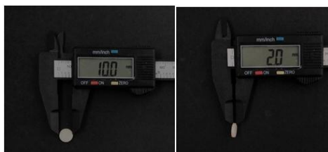
Figure 2: Peek Discs Measuring 10 mm Diameter and 2mm Thickness
