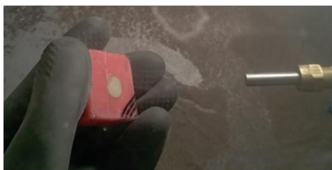
Figure 6: Sandblasting of peek discs using pen blaster with alumina particles
