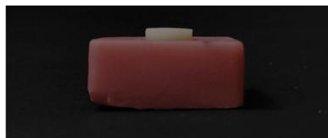
Figure 21: Lithium Di Silicate Discs Placed Over the Peek Samples
