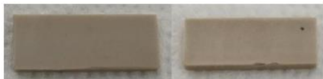
Fig. 2: PEEK specimen after surface roughing to inoculate Candida albicans (right: rough surface, left: bottom)
