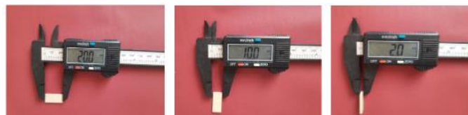
Fig.1: Each PEEK specimen of dimensions 20mm X 10mm X 2mm were milled using CAD-CAM.
