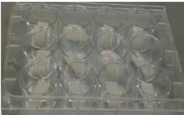
Fig.7: Group C - PEEK with biofilm with 3.8% Sodium Perborate for 15 minutes.
