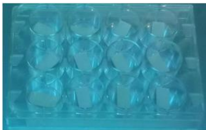
Fig.8: Group D - PEEK with biofilm with UV exposure for 5 minutes.
