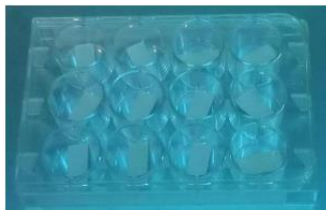
Fig. 9: Group E - PEEK with biofilm with UV exposure for 10 minutes
