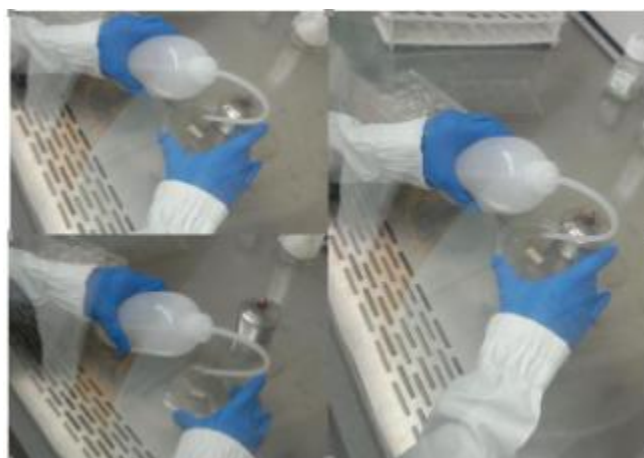
Fig. 4: After incubation with Candida albicans for 24 hours, all the specimens were removed from wells and rinsed gently with PBS 3 times to remove non-adherent cells.
