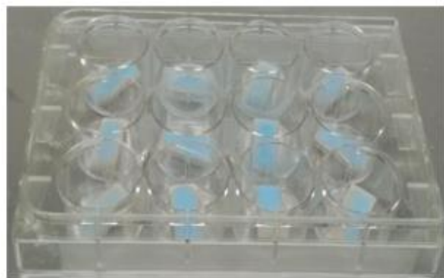
Fig.6: Group B - PEEK with biofilm with 2% Chlorohexidine for 8 hours
