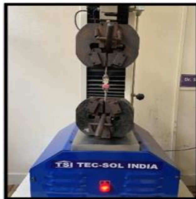
Fig 8: the specimen mounted on the universal testing machine (tec-sol India)
