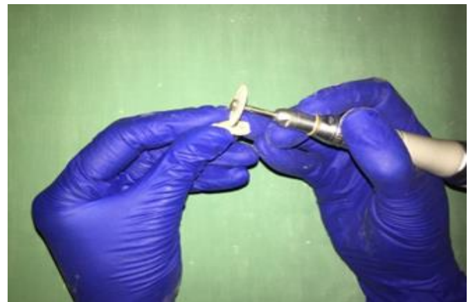
Figure 2: sectioning of tooth
