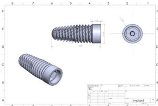
Figure 3: Draft Model of implant with dimensions
