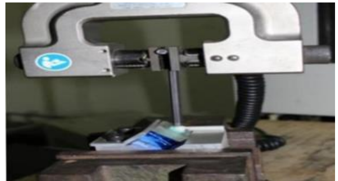
Fig 3: Fracture resistance test using universal testing machine
