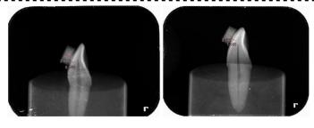
Figure 4: Radiographs to determine substrate thickness
