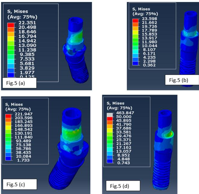
Figure 5: Schematic designs of stress distribution on prosthetic screws of the anterior and posterior loaded and unloaded implants in All-on-4.
