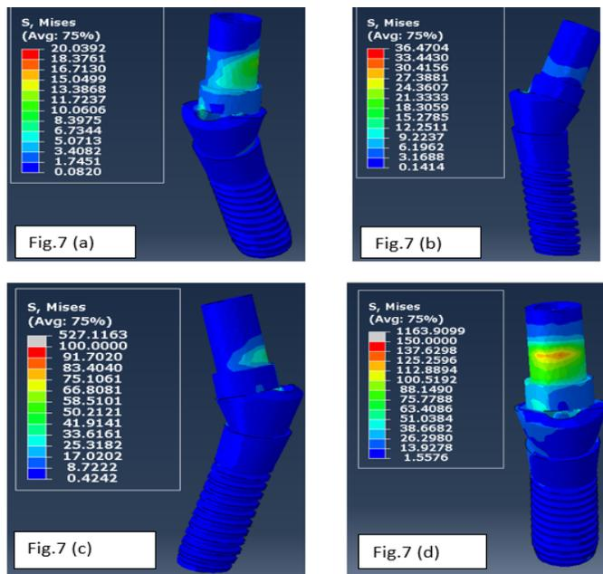
Figure 7: Schematic designs of stress distribution on prosthetic screws of the anterior and posterior loaded and unloaded implants in V4.
