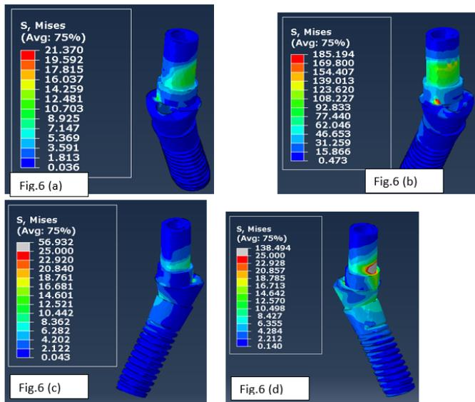
Figure 6: Schematic designs of stress distribution on prosthetic screws of the anterior and posterior loaded and unloaded implants in M4.
