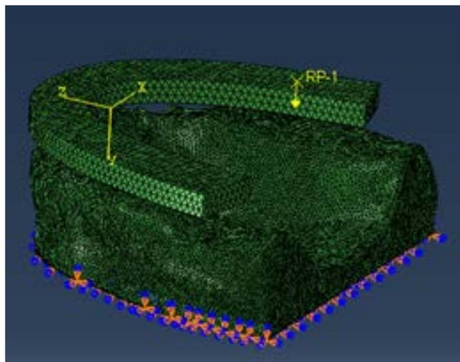
Fig. 4: Application of Load and Boundary conditions in Abaqus software.
