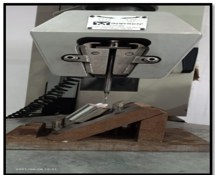
Fig.1: Testing of the specimen for Fracture Resistance
