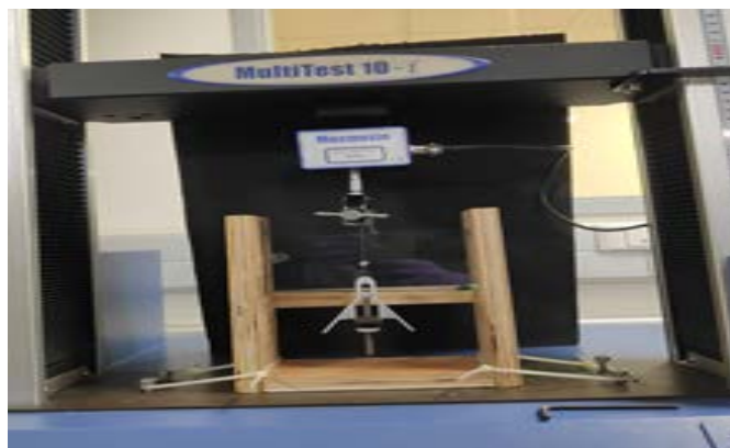
Fig 3: Frictional resistance test setup
