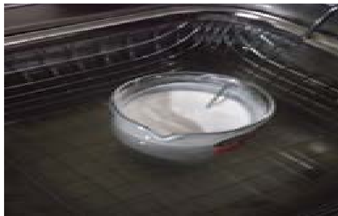
Fig 2: Preparation of ZnO nanoparticle bath in ethanol and ultrasonicator
