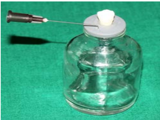
Figure 1: The experimental setup of the collection for extruded debris.
