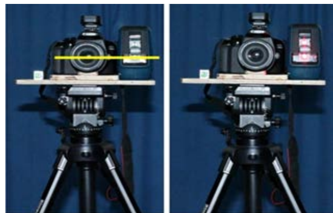
Fig. 4a and 4b: Mounting of wooden base plate with camera and the laser source.
