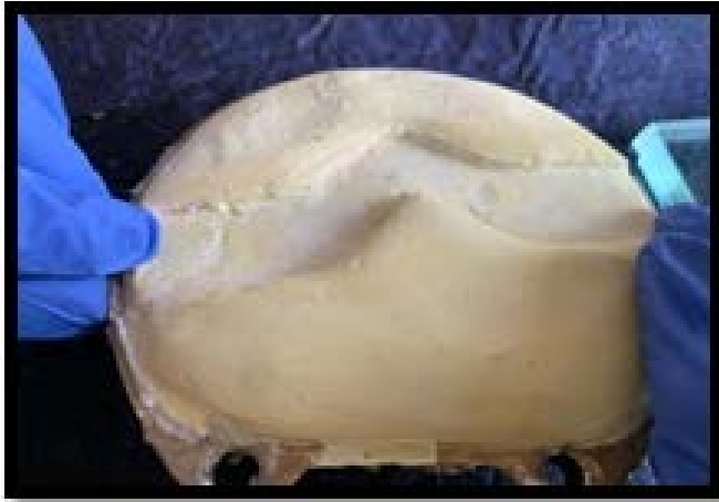
Figure 3 (a): placement of tulle in the mold
