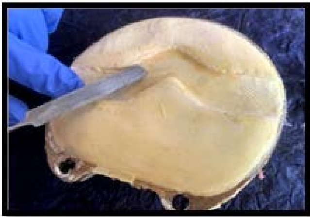
Figure 3 (b) loading of silicone elastomer onto the tulle.
