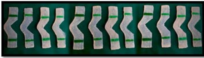
Fig 6 (a) : Silicone samples with tulle marked green
