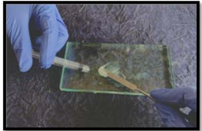
Figure 4: dispensing of 20ppm colloidal silver nanoparticle in silicone elastomer.
