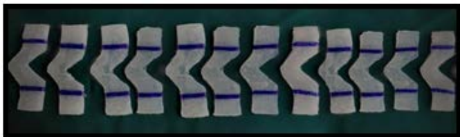
Figure 6 (c): Silicone samples with 1% by weight of polyamide microparticle powder marked green
