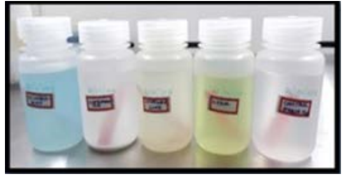
Fig 1: Acrylic strips placed in 5 solutions
