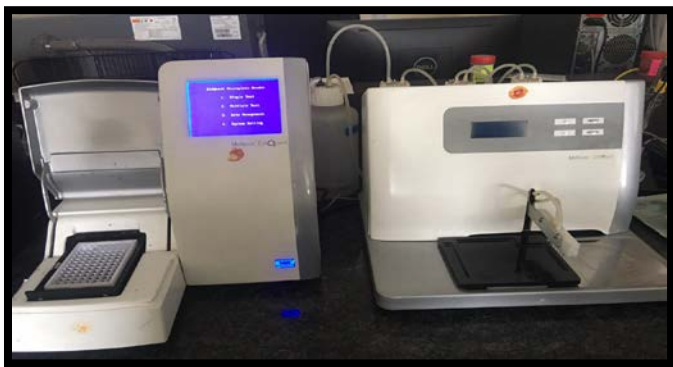
Figure 4: Armamentarium for ELISA Method. Processing of the sample by setting of the wells on the ELISA analyzer
