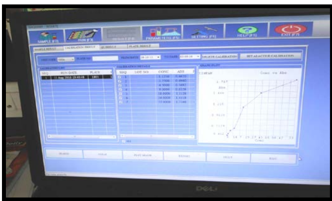
Figure 5: Final result of Micro plate reader as a standard, reference wavelength is 630nm.
